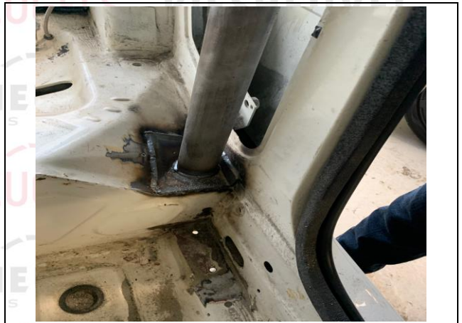
PHOTO 4 MAIN ROLLBAR TO FLOOR ATTACHMENT
