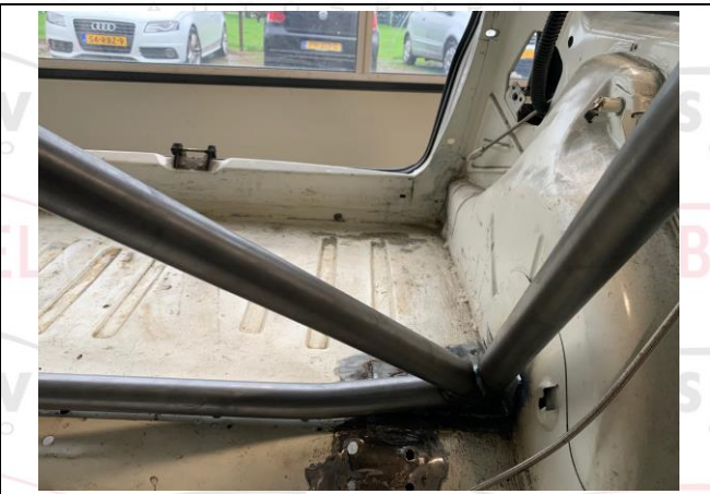
PHOTO 5 REAR BACKSTAY TO BODYSHELL ATTACHMENT
