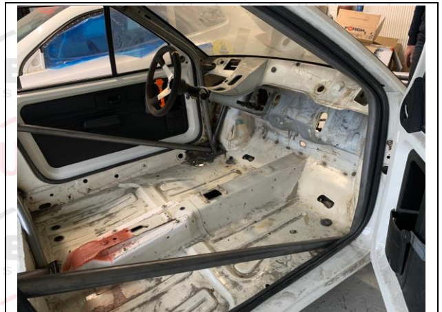
PHOTO 6 FRONT ROLLBAR TO FLOOR ATTACHMENT
